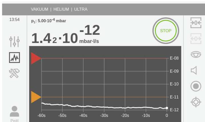
This is a normal behavior of the PHOENIX 4 and shows the real leak rate measurements. The L300i did not show these fluctuations in the low decades. The L300i had a different calculation, which “softened” these fluctuations, and the resolution of the display was too low to show these very small fluctuations.
