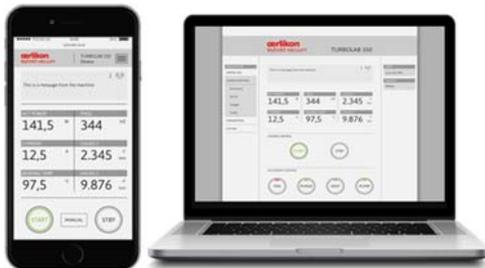
Webserver "browser based" Control/Monitoring/Configuration Tool for mobile & desktop browsers and TURBOLAB Widget, the PC software tool for monitoring multiple TURBOLAB's status & key values.
